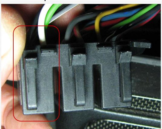
Cut the connector shell along the line shown.
